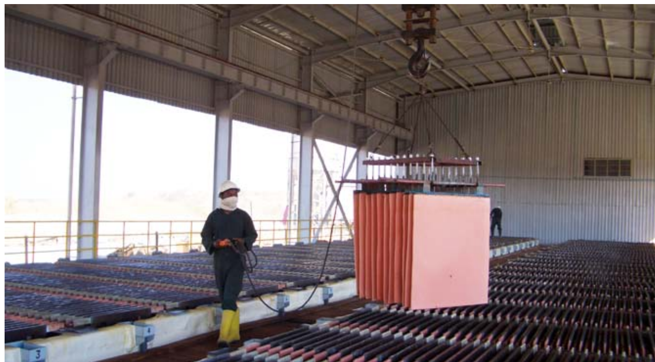
Copper produced in the extraction and electrowinning workshop
